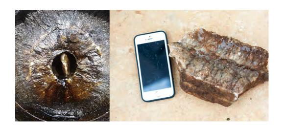
CHEMICALS TO INHIBIT THE SCALE AND PARAFFIN AND USING ACIDS TO CLEAN THE FLOWLINE AND OIL WELLS. EVEN BY DOING THIS, THE SCALE STILL PLUGS OFF THE FLOWLINE AFTER 2-3 MONTHS.
